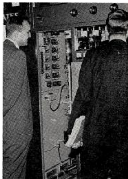
Couple of broadcasters look over innards of Townsend Associates 50 kw UHF television transmitter.
